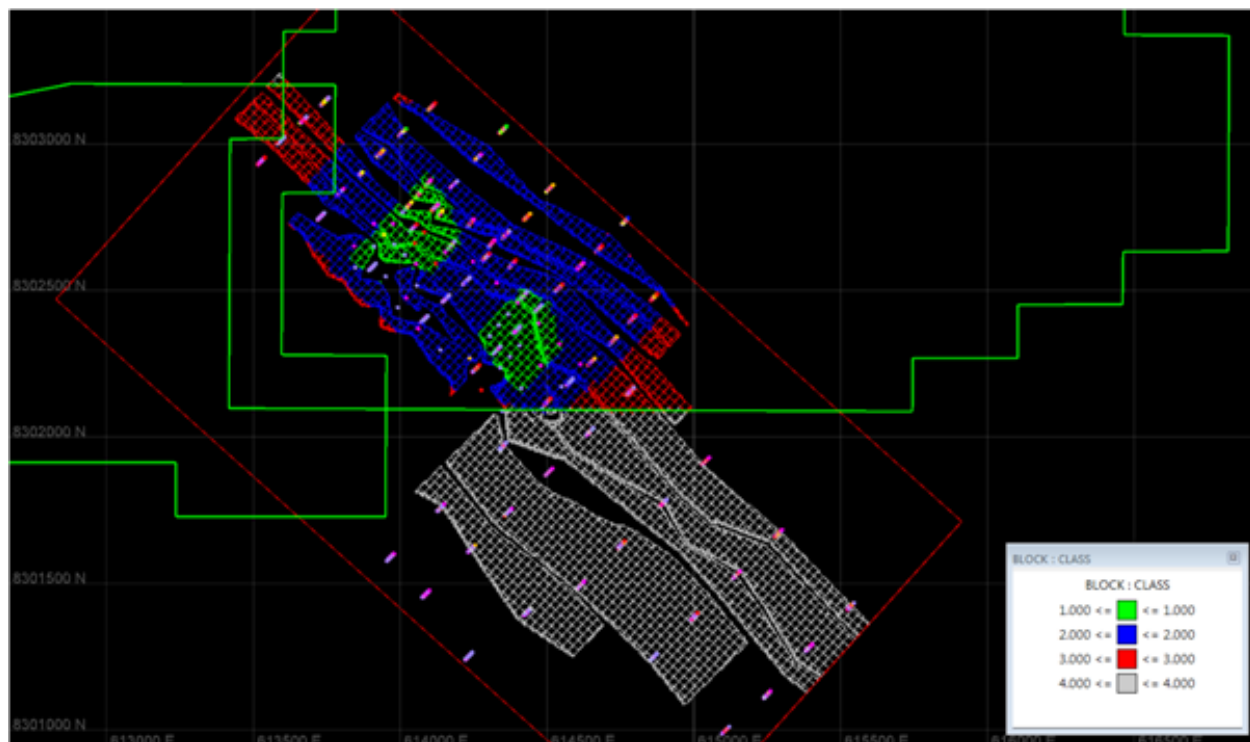
Figure 1: Plan view of Limeco's MRE as reported by Golder in 2017; Class 1 = Measured (green), Class 2 = Indicated (blue), Class 3 = Inferred (red) and Class 4 = Exploration Target (grey).
