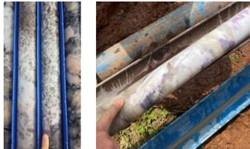
Recent core with visible spodumene (left) and spodumene & lepidolite (right)
