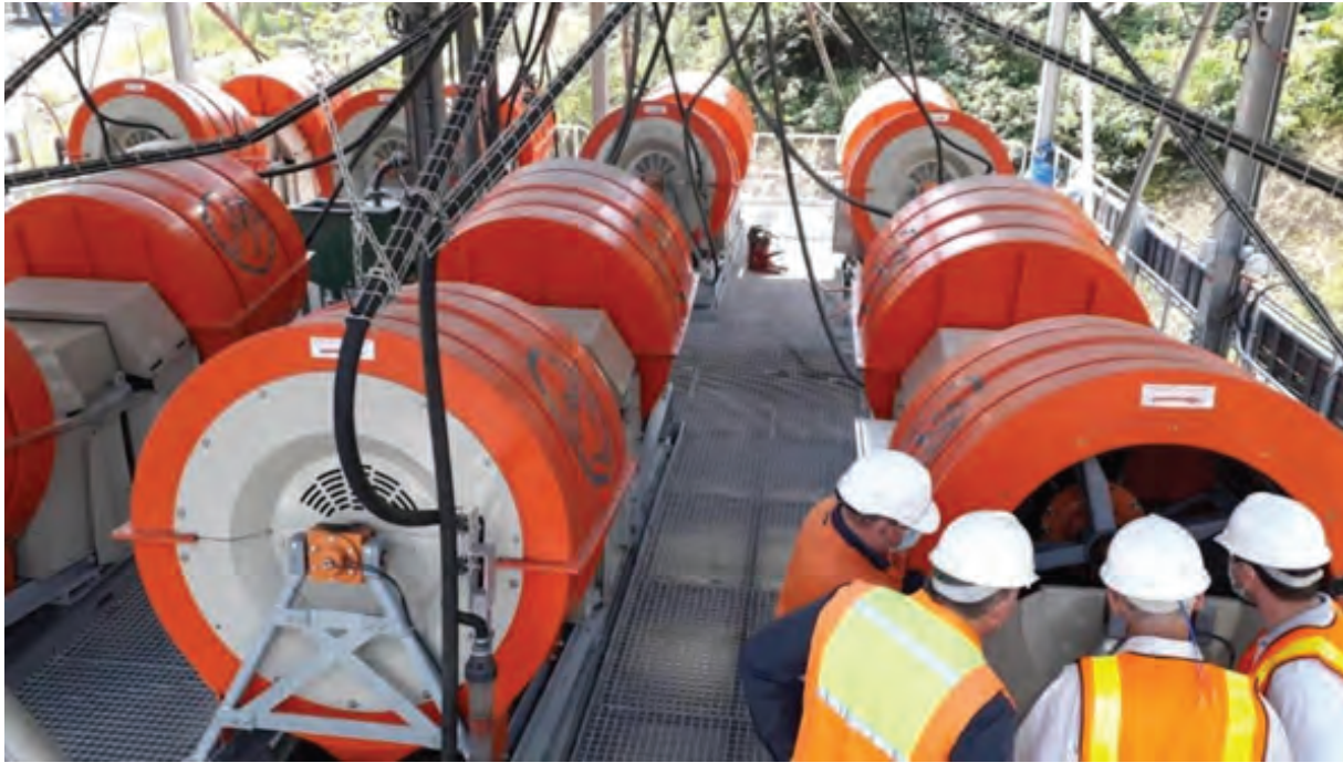
Figure 8: View of the seven C900 units operating at Alphamin Resources' Fine Tin Project (Source: Gravity Mining, 2021).
